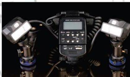
**Figure 6:** A typical twin flash system
