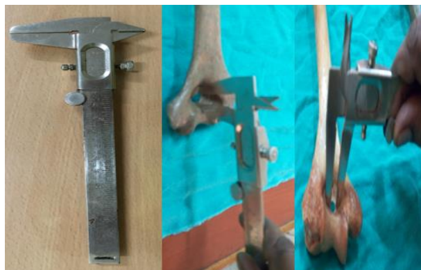
Fig 2: Measurement of vertical and transverse diameter of STF using the vernier calipers
