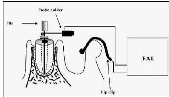
**Fig. 1: Circuit for electronic determination of working length**
