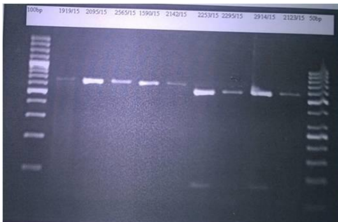
Fig. 2: Detection of V domain mutation: Mutation noticed in 1919/15, 2095/15, 2565/15, 1590/15, 2142/15 (628 bp)
