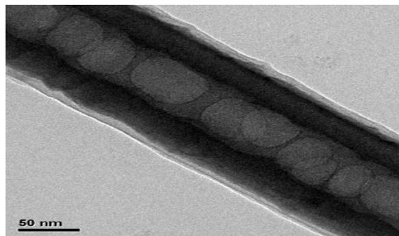
**Fig. 8: TiO<sub>2</sub> nanotube as drug delivery system**
