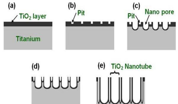
Fig. 6: Electrochemical anodization
