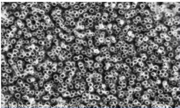
Fig 5: Cluster of TiO<sub>2</sub> tubes
