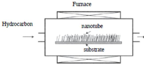
Fig. 2: Seeding method of carbon nanotube synthesis
