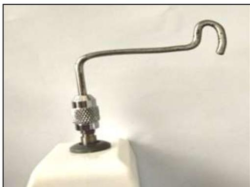
**Fig. 4: Hook modification of push and pull gauge**
