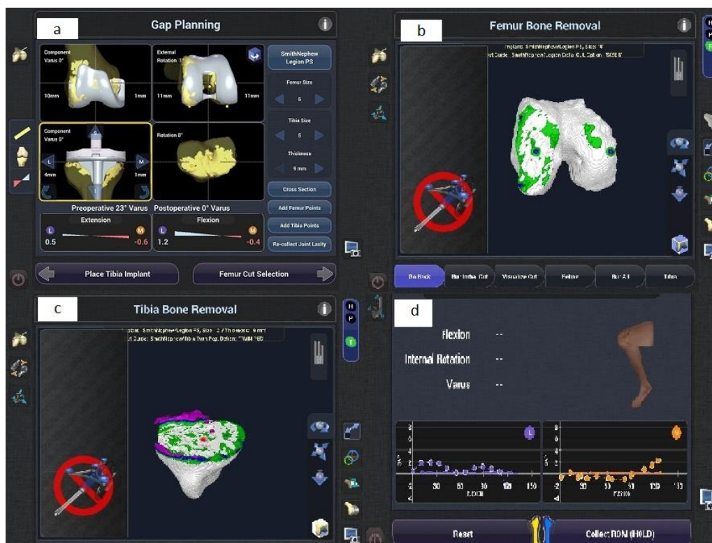
Fig. 2 a): Gap planning screen shows flexion /extension graph balancing; b): Femoral distal cut, minimal medial condyle cut c): Proximal tibial cut; d): Post op graph balanced throughout knee range of motion
