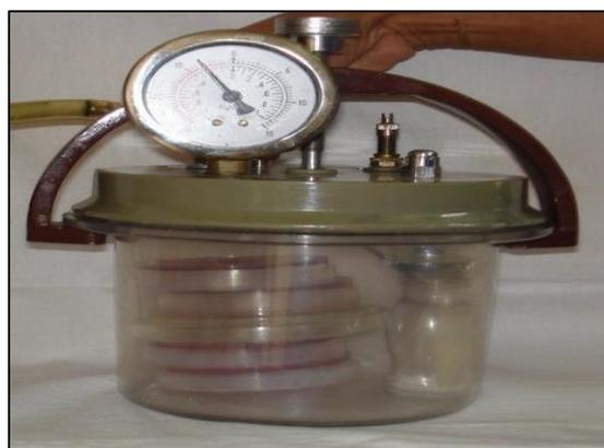
**Fig. 5: Anaerobic glass jar and incubator for bacterial culture**
