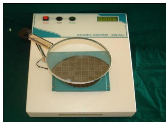
**Fig. 6: Colony counting unit and magnifier for colony count**
