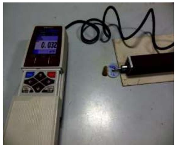
**Fig. 5: Surface roughness tester. (Mitutovo, Japan, SJ 210)**
