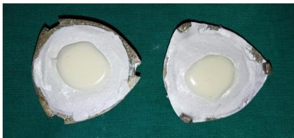
**Fig. 13: PMMA packed into dewaxed mold**
