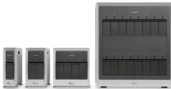
Fig. 2: Gene Xpert instruments with 1, 2, 4 and 16 modules
