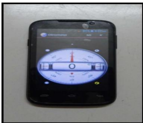
Fig. 1: Clinometer application on smart phone
