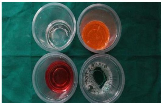
**Fig. 1: Wires in distilled water, artificial orange, mouthwash, wine**
