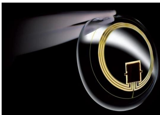
**Fig 15: SENSIMED Triggerfish contact lens**
