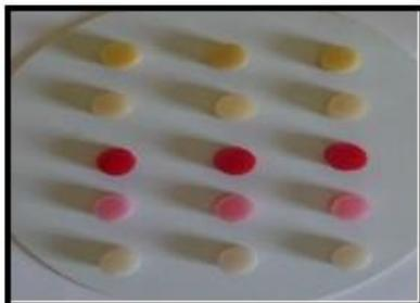
**Fig. 4: Samples of different waxes used in flow, hardness and accuracy test**
