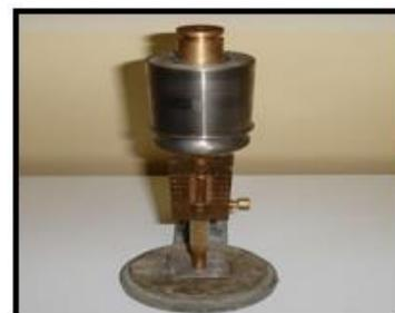
**Fig 2: Vicat apparatus after modification**
