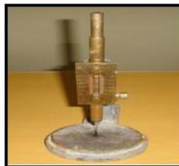
**Fig 1: Standard Vicat apparatus**
