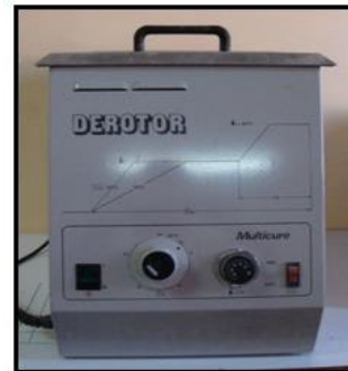
Fig. 5: Controlled water bath
