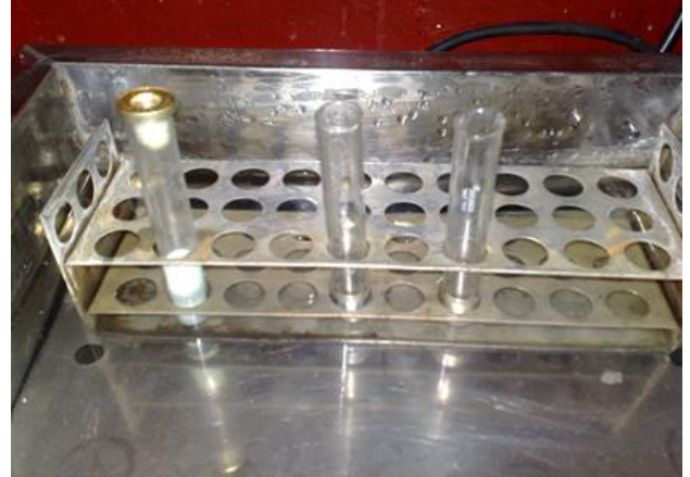
Fig. 4: Methylene blue reduction test
