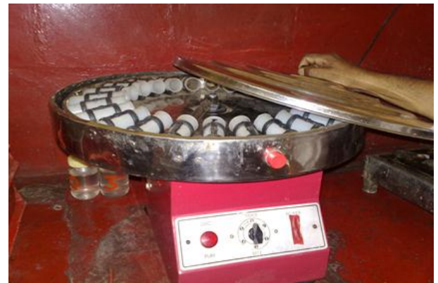
Fig. 5: Centrifugal machine to do the fat test
