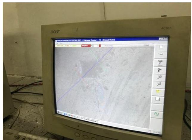
Fig. 2: Measuring the indentation made on composite
