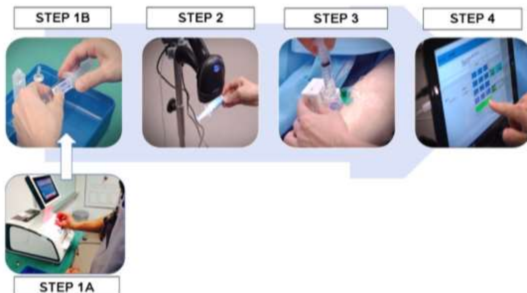
Fig. 2: The AVOID-error system drug administration workflow; Step 1A -1B: The end user scans the drug ampoule and prints the syringe label using a label printer OR uses Prefilled prelabelled syringes; Step 2: The system mandates scanning the syringe-label using the device scanner prior to drug administration. The scan produces an audio-visual cue consisting of drug name and concentration; Step 3: On successful completion of Step 2, the AVOID patient IV device unlocks and allows injection of syringe into the drug administration port; Step 4: After drug injection, the end-user enters administered drug amount into AVOID-error system
