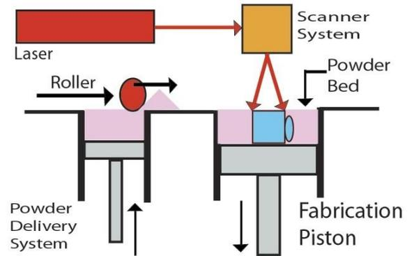
**Fig. 3: Selective Laser Sintering**
