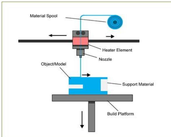
**Fig. 2: Fused Deposition Modelling**
