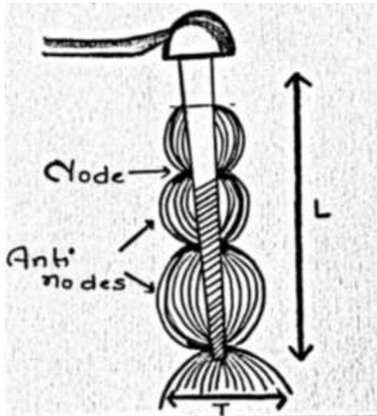
Fig. 8: Oscillation of Ultrasonic Instrument
