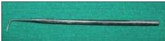
Fig. 2: Modified probe for holding wire
