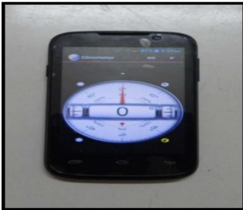
Fig. 1: Clinometer application on smart phone
