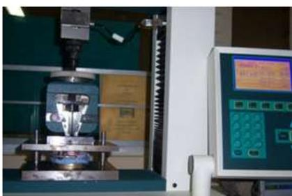
Fig.4: Impression made on universal testing machine
