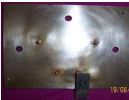
Fig.3: Custom tray positioning plate
