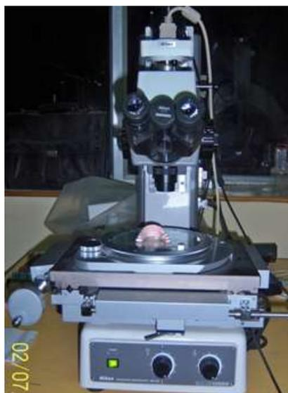
Fig.7: Toolmakers microscope
