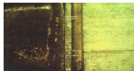
Fig. 11 & 12: Microscopic view of coping fabricated with accelerated casting technique using ringless method showing marginal discrepancies (Group 4)
