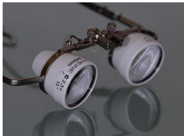
Fig. 2: Fixed compound loupe, adjustable only in the inter-pupillary distance (Galilean Principle)
