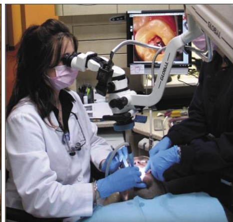
Global G-6 SOM with an enhanced metal halide illumination system.
